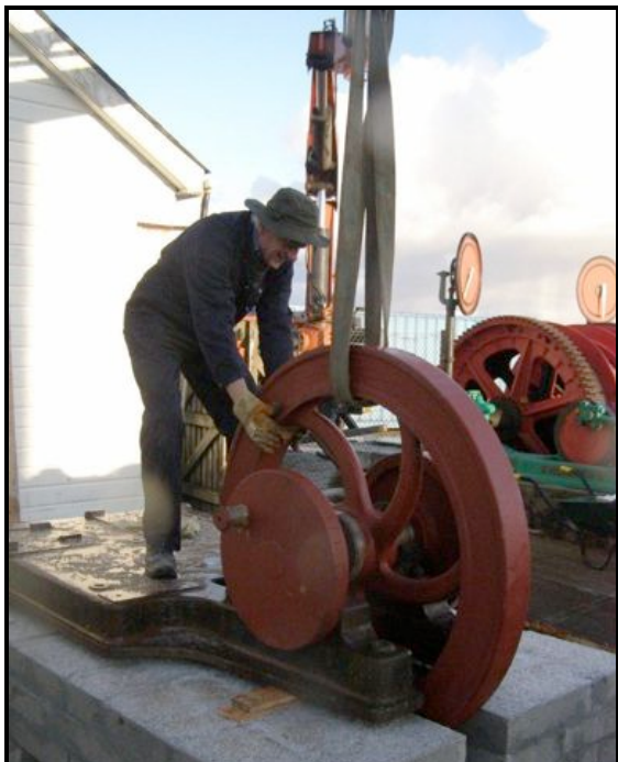
David Blight checking freedom of movement after the flywheel had been positioned.
