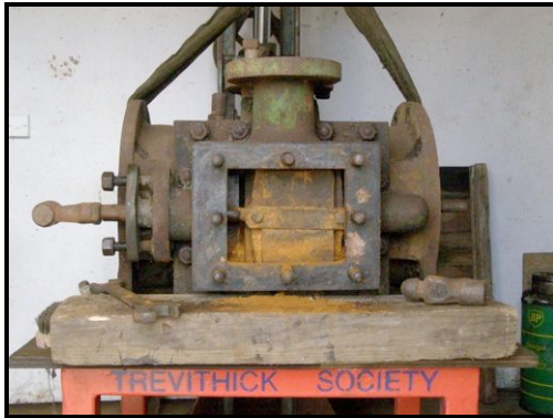
The steam side compressor piston before renovation
